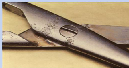
This tool shows evidence of pitting and should undergo repair.
