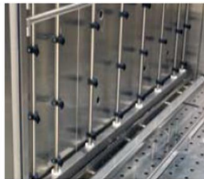
Lateral washing system and multiple drying ports.
